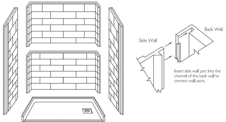
**FEATURES** Dimensional Tolerance  $\pm \frac{3}{16}$ ". Dimensions needed for site preparation should be measured from the unit. American Bath Group assumes no responsibility for preparatory work.
