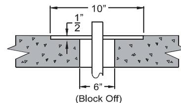
Note: Unit will not install properly if framing pocket is not square and of proper size. The dimensions shown in the FRAMING DIAGRAMS are 1/4" larger than the size of the shower pan. This product is manufactured to tight specifications. The 1/4" over sizing is for maneuvering and installation ease. If 1/4" over is not reasonable, sizing closer to the product actual dimensions is allowable.
